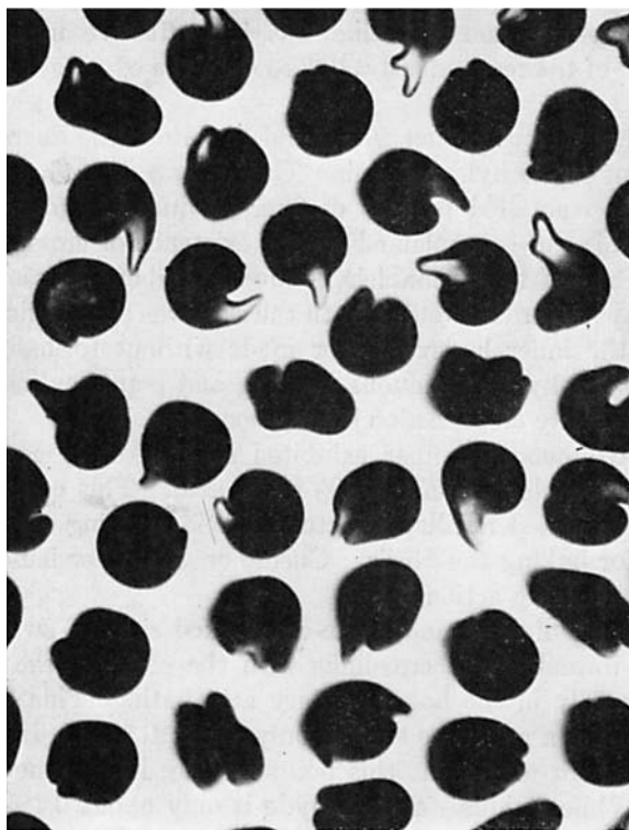
Fig. 13. Photomicrograph of cross section of fiber made at 260% stretch with formaldehyde in the spin bath. Stained, 880 \times .
